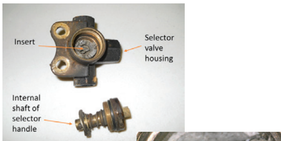
Figure 2. Fuel selector valve housing and section of selector handle (above) and fuel selector insert with fractured pieces (right).
