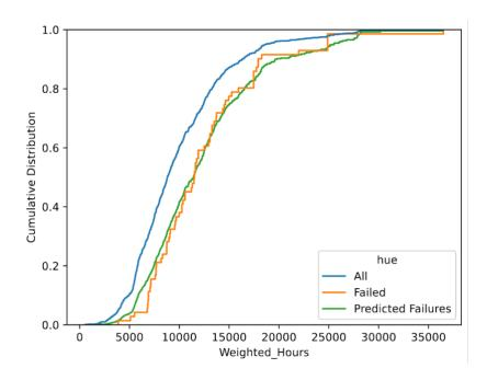
Here, we see that by simulating failures under an assumed model of random occurrences (e.g., hard landings), the number of inspection failures predicted almost perfectly lines up with those seen in practice.
