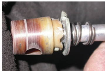
Figure 5. Plug cock showing discoloration, scoring, wear, debris, and a worn detent.
