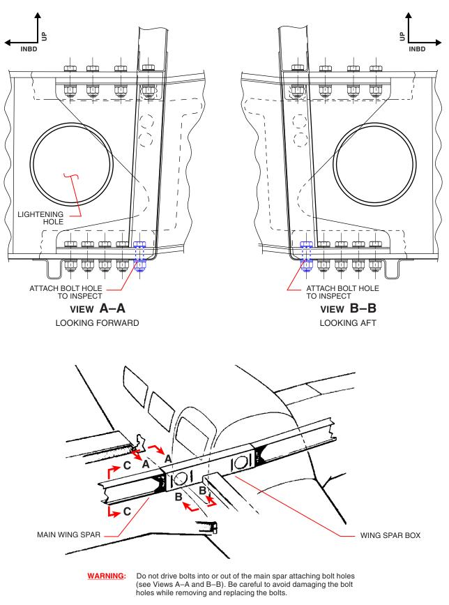
Figure 1, Sheet 1 of 2 Typical Main Wing Spar Attach Bolts and Spar Cross Section (Right Wing Shown)
