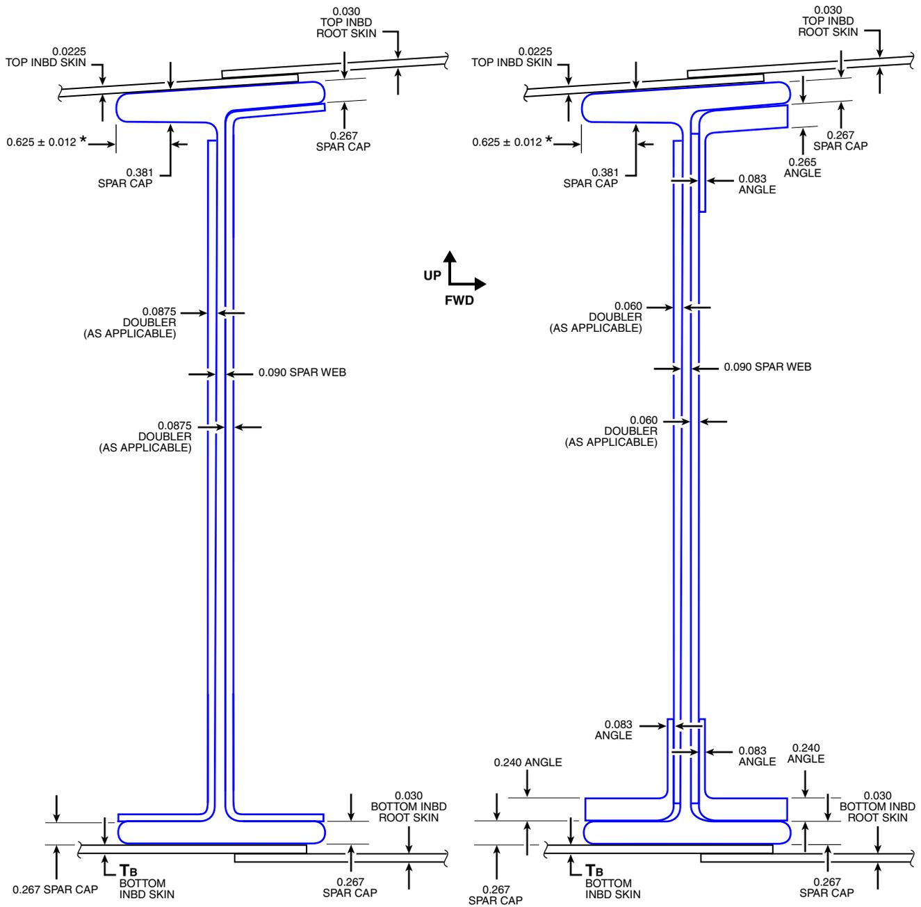
**NOTE:** The minimum allowable dimensions are shown in View A-A and B-B, except as denoted by \*.
