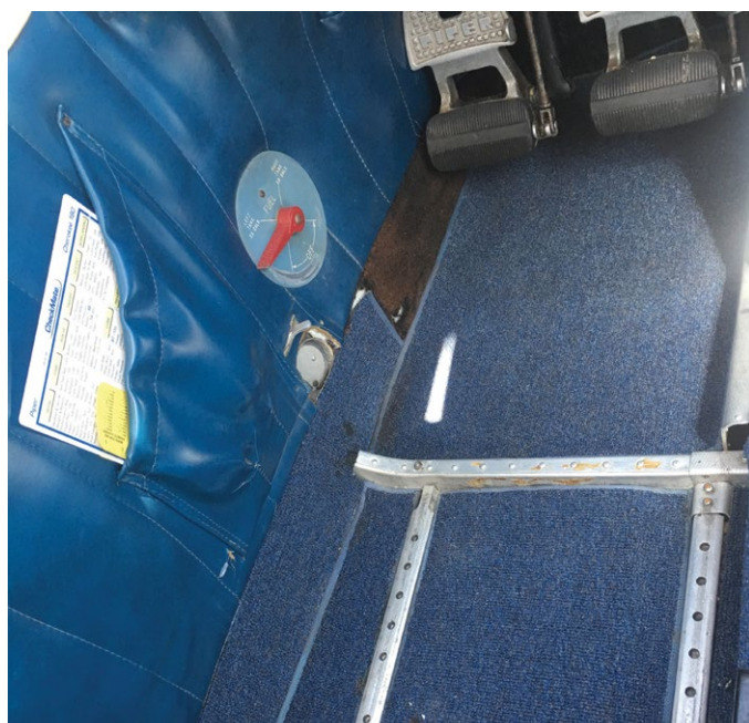
I even replaced the fuel selector with a modern version. The original one worked fine, it just looked antiquated.
