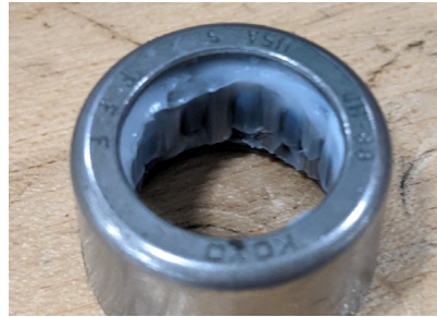
Greased Bearing Before Installation
